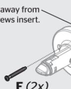
**E** Push up on lever base while tightening screws to keep latch horizontal and centered.
