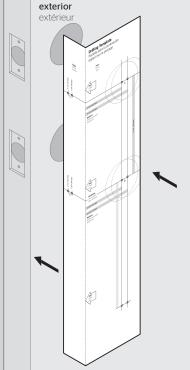
B If you already have the bottom hole drilled in your door, confirm that it aligns with the bottom hole in the template. If it does not align, drill a new hole in step 3.
