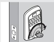
C Close the door. Insert and rotate the key to lock the door. Ensure that the door locks smoothly.
