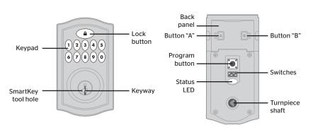
Note: When the cover is removed, the turnpiece shaft can be used to manually lock and unlock the door.
