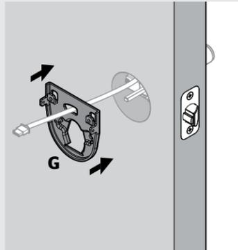
**C** Secure mounting plate with supplied screws.
