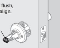
**D** Tip: Pull lever slightly away from door to see where screws insert.
