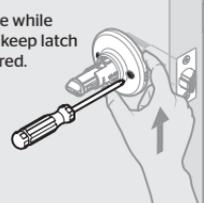
**F** Install interior lever and tighten pre-installed set screw.
