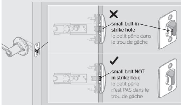
If latch is loose in the strike, adjust the strike tab so it grips the latch bolt better when the door is closed.
