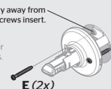
**E** Push up on lever base while tightening screws to keep latch horizontal and centered.
