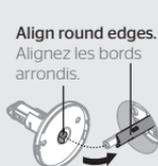
**C** If lever base won't sit flush, rotate turnbutton to align.
