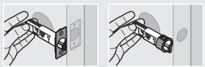
**B** If the latch holes are centered in the door hole, no adjustment is required. Proceed to step 4.
