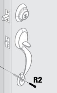
**17 Determine required screws for mounting knob or lever**
