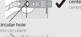
**B** If the semi-circular hole in the latch is centered in the door hole, no adjustment is required. Proceed to step 3.
