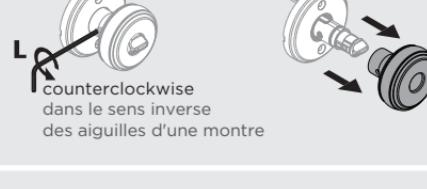
**B** Press in latch bolt while installing exterior knob.
