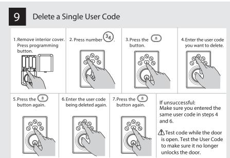
If a button is not pressed within 5 seconds, the system will time out, and you will need to
