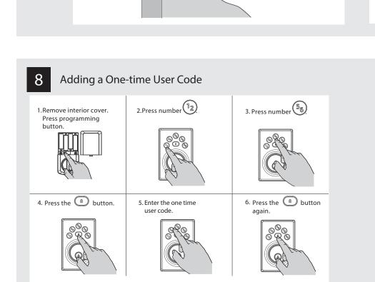
Up to 2 One-time User Codes can be saved. One-time User Codes should be 4 to 8 digits in length.
